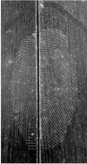
FIG. 7—Mark treated with white powder on treated wood aged one month (both sides).
