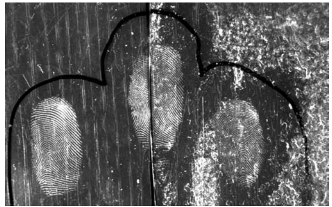
FIG. 14—Left side cyanoacrylate/stain only; right side sprayed with iodine-benzoflavone, then cyanoacrylate/stain (viewed under white light).
